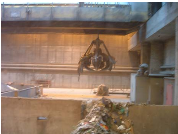
From there, the MSW is picked up by a grapple hook and placed in a shredder.
