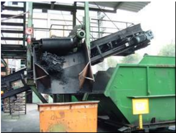
The ferrous metal contained in the solid residue is extracted with a magnetic separator and conveyed into a small bin.
