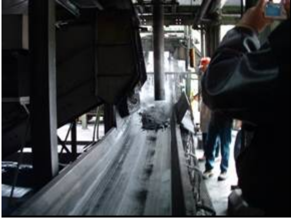
The char mixture is dumped onto the conveyor belt.
