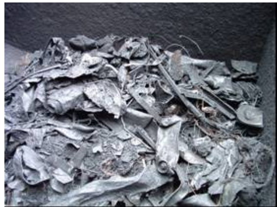
The ferrous metal contained in the solid residue is extracted with a magnetic separator and conveyed into a small bin.
